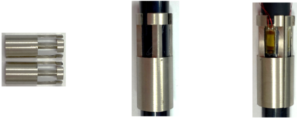
Figure 6.2.2: A custom made strain gauge attachment to help ensure consistent strain-gauge placement. This attachment fitted around the sample of each posterior strut to indicate the location and orientation for each strain gauge.
