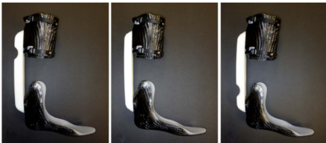
Figure 3.4.4: The 3 selective laser sintered posterior struts used in studies by Ranz et al. and Esposito et al. examining the changes in gait during walking and running, as the bending axis changes [39, 54]. Image reproduced with permission from the rights holder, Elsevier [54]
