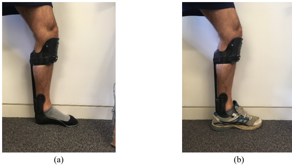
Figure 5.3.2 PD-AFO as worn by the subject (a) without and (b) with trainers
