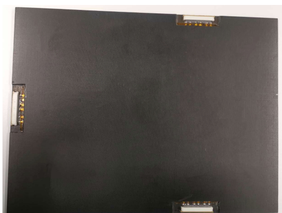
Figure 6.3. Schematic of the panel with embedded PZT transducers after trimming
