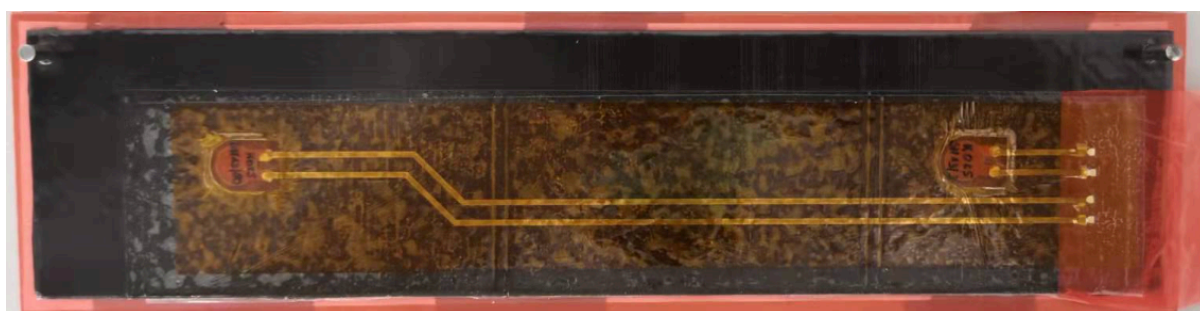
Figure 3.10. Examples of an embedded diagnostic film with PZT transducers.
