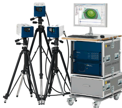
Figure 2.9. Schematic of the PSV-500-3D Polytec 3D Scanning Vibrometer [114].
