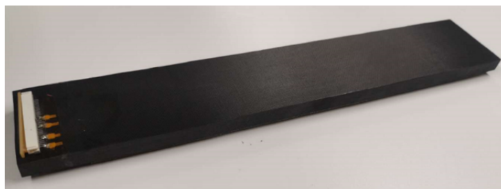
Figure 6.33. The 9 mm coupon with middle-embedded ending terminals and a connector.
