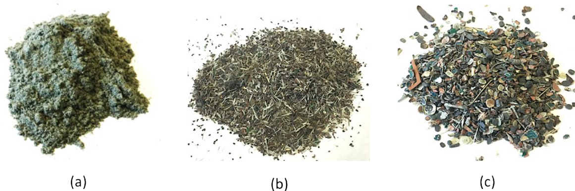
Figure 3.9: PCB samples obtained after milling; (a) \leq 150 \mu\text{m} , (b) 150\text{-}710 \mu\text{m} , (c) 710\text{-}2000 \mu\text{m} .
