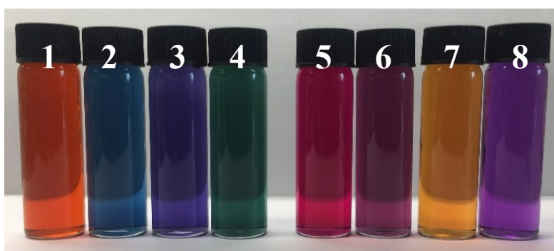
Figure 62. Photograph of DX-IDF copolymers [2-4] and DX-IDT copolymers [6-8] dissolved in DCM at equal concentrations, demonstrating the spectrum of absorption wavelengths, resulting in the varying coloured solutions.
