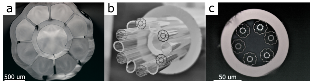
270 271 Fig. 9. (a) An optical micrograph of a microstructured resonator drawn using SSED. (b) A photograph of a stack 272 incorporating the microstructured resonators, ready to be drawn into canes using another SSED step. The stack has a 273 25 mm outer diameter. (c) An optical micrograph of an ARF with microstructured resonators.
