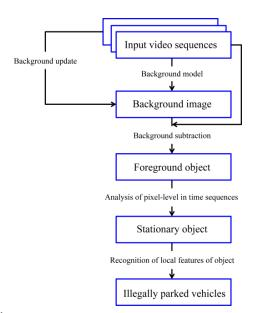
Fig. 1. System architecture of the proposed system.
