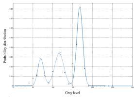
Fig. 2. Probability distribution of the gray value of a certain pixel point in the time sequence with three Gaussian curves.
