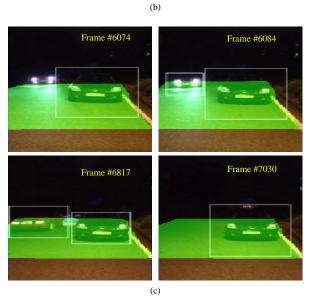
Fig. 6. Some test results of the proposed illegally parked vehicle detection algorithm. (a) Highway: morning. (b) University road: evening. (c) Urban road: night.
