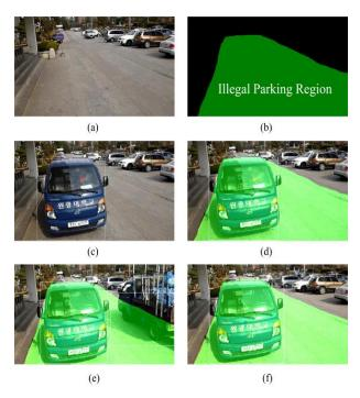
**Fig. 5.** Results of the proposed illegally parked vehicle detection algorithm. (a) Background image. (b) Illegal parking region model. (c) Vehicle parking detection in  $450^{\text{th}}$  frame. (d) Vehicle parking detection in an illegal parking region in  $450^{\text{th}}$  frame. (e) Vehicle parking detection in an illegal parking region in  $8120^{\text{th}}$  frame. (f) Vehicle parking detection in an illegal parking region in  $9105^{\text{th}}$  frame.
