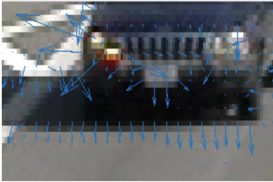
Figure 5.3: shows the concept of the Optical Flow algorithm's purpose. The Optical Flow allows to track objects between frames, estimate their current velocity to detect the position in consecutive frames so to track their movement. An object at position (x,y) will undergo a displacement and be at position (x+dx,y+dy) in the next frame at some time later. The constriction will be to say the intensity of the object will be constant.
