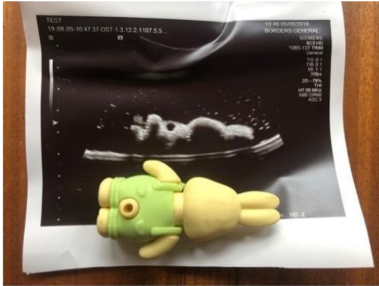
Figure 3-1. Ultrasound appearance of rabbit shaped rubber eraser contained within a water filled rubber glove. Ultrasound image captured by Alexandra Viner using Fujifilm SonoSite M-Turbo ultrasound machine. Photo by Alexandra Viner.
