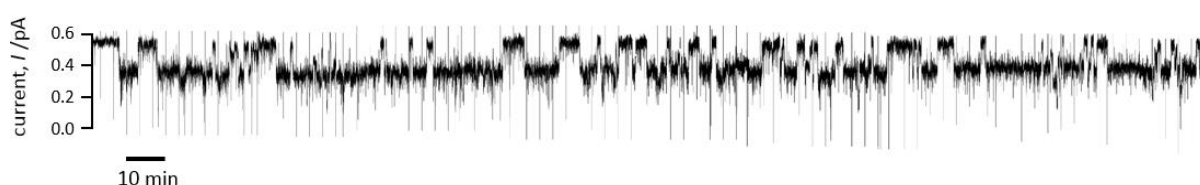
Figure 5.3 Real-time current trace during transmembrane rolling circle amplification
