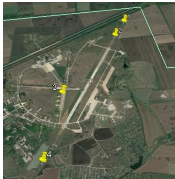
Figure 6. Control points for aircraft noise measurements at Zaporizhzhia International Airport.
