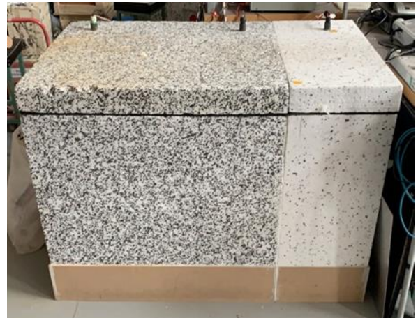
Figure 3 Hot Box apparatus
