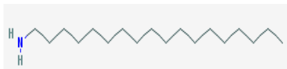
Figure 1.15: Chemical structure of Stearylamine (Octadecan-1-amine; source: https://pubchem.ncbi.nlm.nih.gov/compound/octadecylamine#section=Top ).
