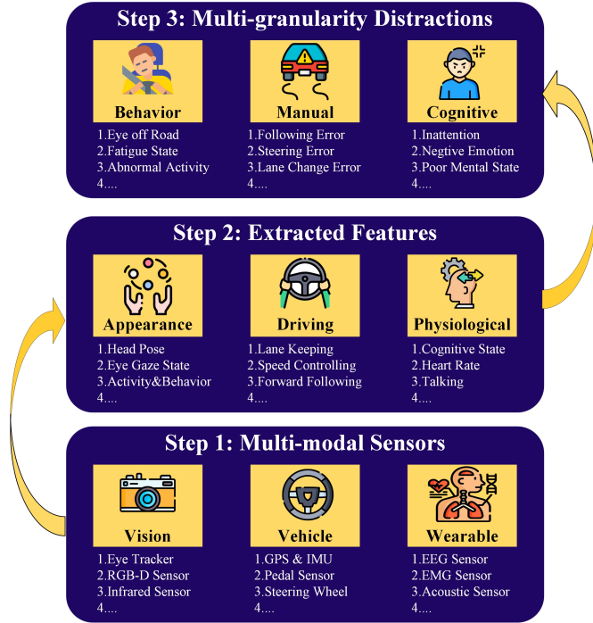
Fig. 5. General framework of driver distraction detection.
