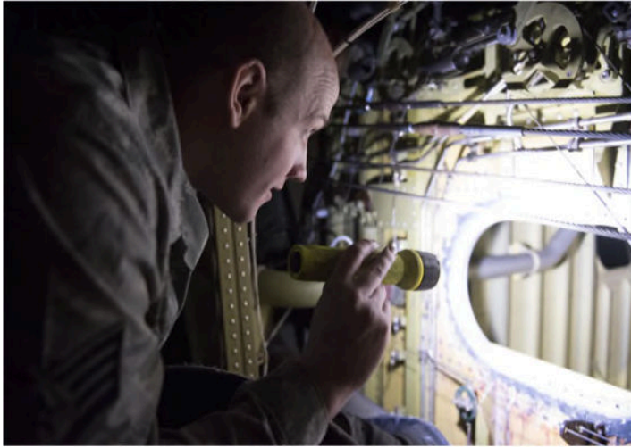
Figure 2. Engineer using flashlight to inspect fuel tank and personal in fuel tank wearing protective equipment during inspection
