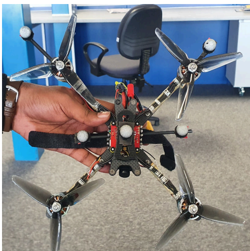
Figure 6: Symmetrical Structure - SY.
