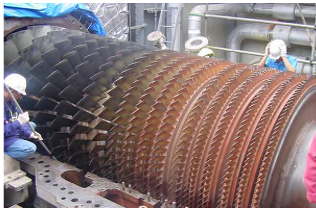
Figure 1 Front stage fouling of a multi-stage compressor [9]
