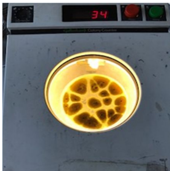
Figure 6.4 Colonies of A.flavus being counted using a colony counter.
