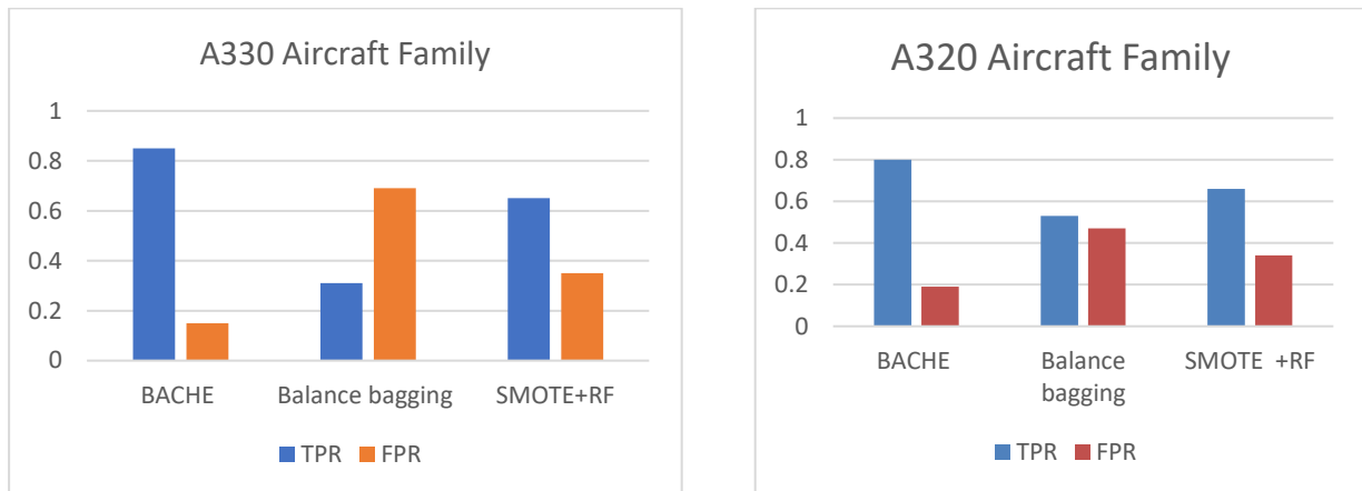
Figure 5- 5 The average overall performance of each algorithm on the two aircraft families (A330 and A320)
