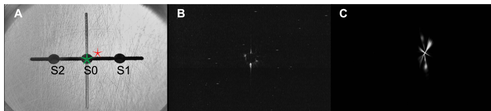
Fig. 11. Slit-jaw images obtained during X-ray testing at the XRCF. (A) Modified slot fully illuminated with white light. Positions along the slot, S2, S0 and S1 are labeled and correspond to results shown in Fig. 18. (B) Edges of the guide laser illuminates edges of slot at position S0. (C) Guide laser image is fully visible while pointed off of the slot. The locations of the guide laser pointed on the center of the slot and off the slot relative to the fully illuminated slot are shown (green and red star, respectively).
