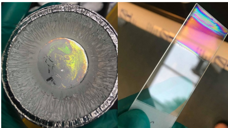
Figure 7.11 Structural colour of deposited SNPs film (SMS 35 functionalised with HMDZ)
