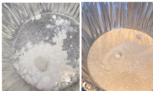
Figure 7.6 water drop wettability test; (a) un-functionalised Aerosil 200, (b) HMDZ functionalised Aerosil 200
