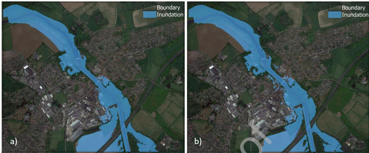
Fig. (16): Hydrograph 7 Maximum Depth across flood events, with a threshold of 0.3m to highlight inundation, (a) Maximum Inundation calculated by LISFLOOD-FP, and (b) Maximum Inundation calculated by GP emulator.
