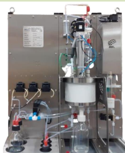
Figure 5: CCF20DD Continuous Carousel Filter with Re-slurry, Dissolution and Drying unit
