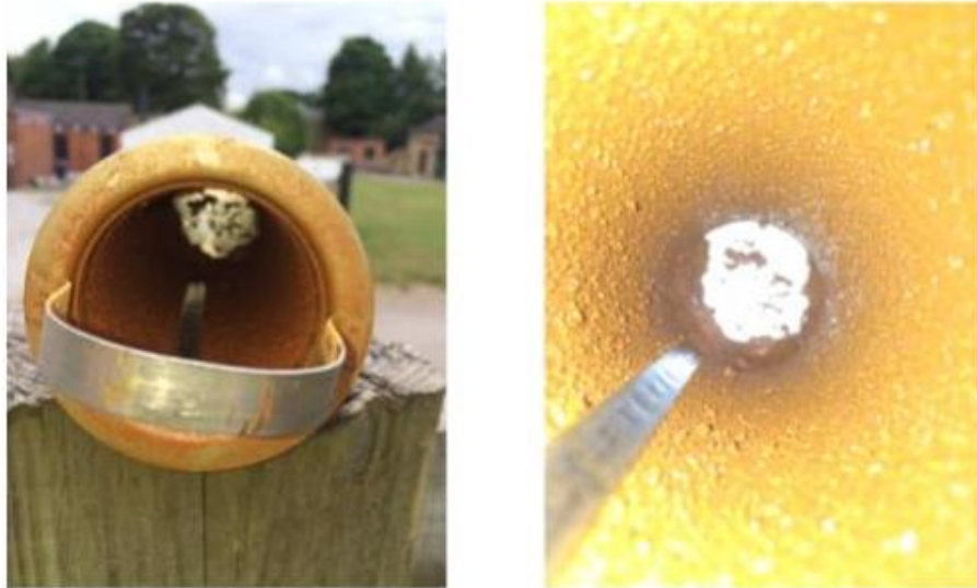
Figure 20 Caphouse filter after dousing of sodium dithionite
