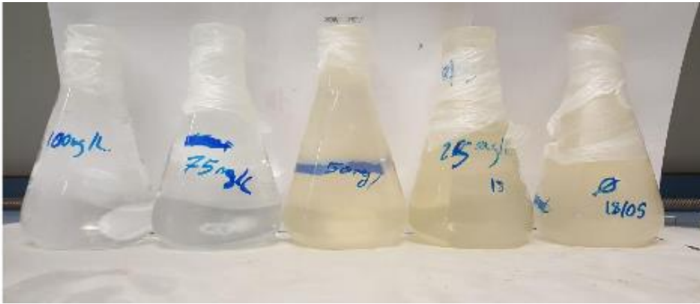
Figure 22 Mine water response to the addition of different doses of sodium dithionite. Concentrations of 75 and 100 mg/l keep the iron completely dissolved as Fe^{2+}
