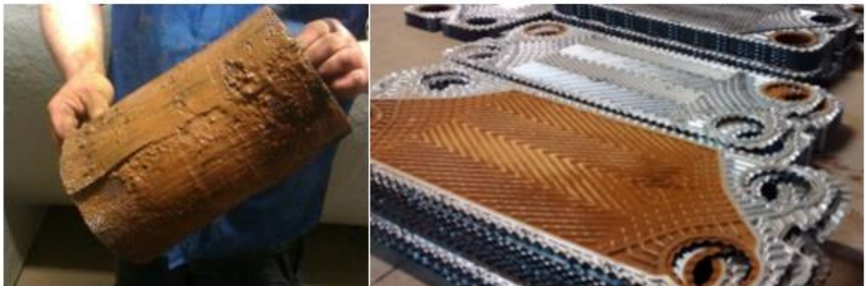
Figure 21 Ochre deposition in a filter and in a plate of the exchanger in Barredo
