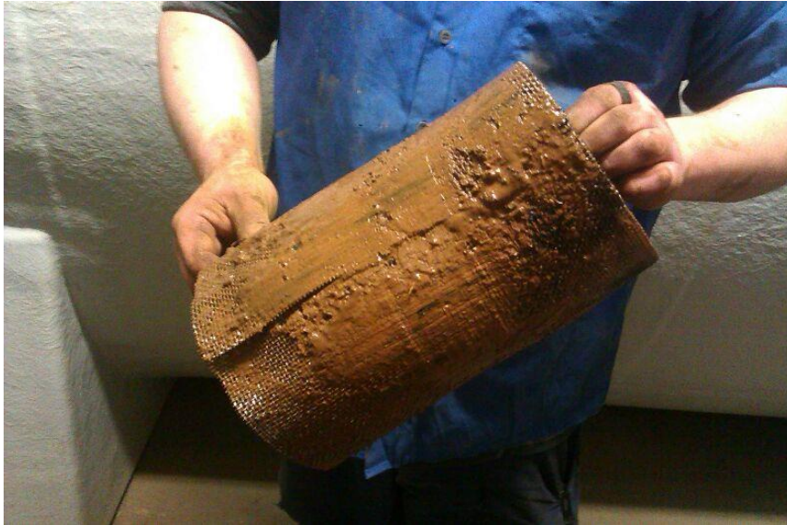
Figure 57. Filter full of iron
