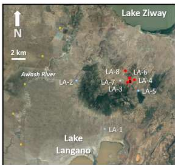
Figure 1: Satellite image of Aluto-Langano volcanic complex (from Google Earth) showing surface water features and location of geothermal drilling activity (coloured circles). Red- productive wells; Green- reinjection well; Blue- non-productive wells (all from Teklemariam & Beyene 2001); and Black with red outline- newly-drilled directional wells (from Biru 2016).
