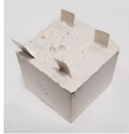
Fig. 7. Pure geopolymer block with protruding electrodes.
