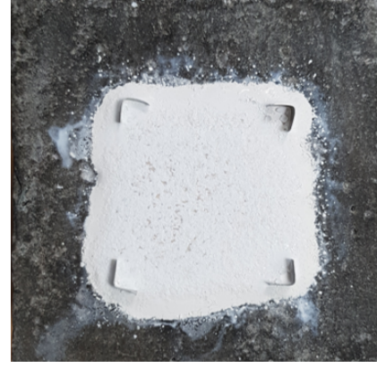
Fig. 2. Small spray-coated geopolymer patch.
