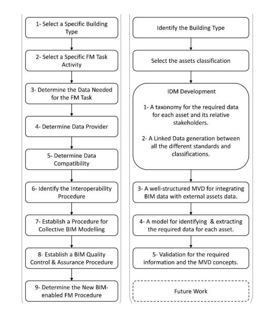
Figure 1: Two framework by Pishdad-Bozorgi et al. (2018) and by Farghaly et al. (2018) to effectively integrate data between BIM and AM systems.
