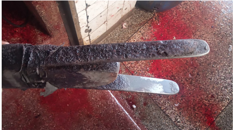
Fig 5. An image showing the dirty and corroded electrodes on the stunning device.
