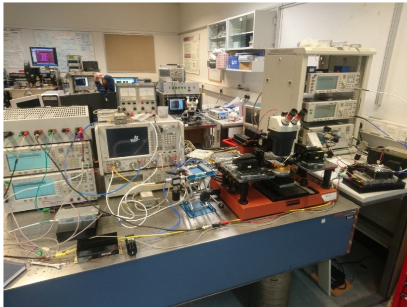
Figure 6.1 - Load Pull measurement system deployed at Cardiff University based on PNA-X.
