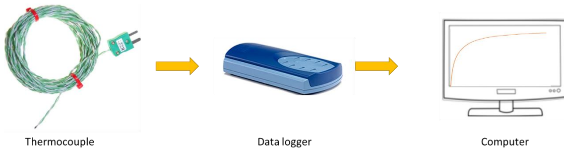
Figure 3.27: Temperature measurement, monitoring and recording sequence.
