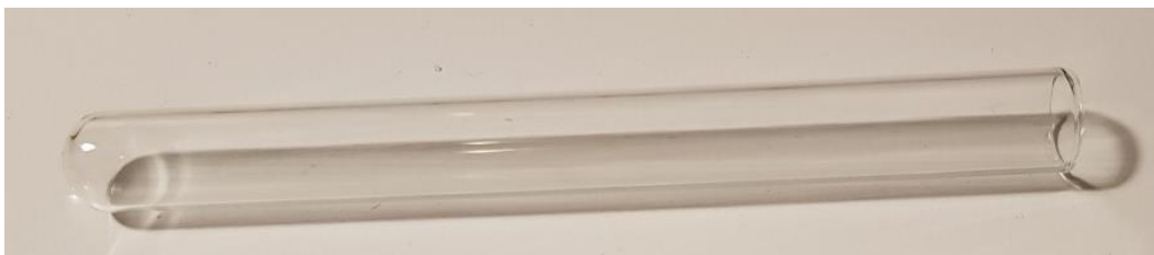
Figure 6.2: borosilicate glass tube that was used to cover the copper rod.
