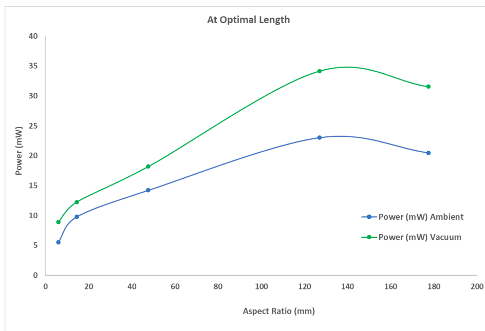
Figure 4.25: TEG modules theoretical power output vs. the aspect ratio in ambient and vacuum environment at optimum thermoelement length.
