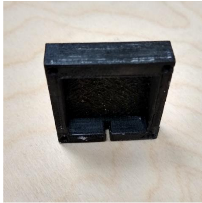
Figure 6.5: The 3D printed cover for the copper absorber end for insulation experiments.
