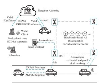
Fig. 19: The blockchain-based AD Dissemination framework [230]
