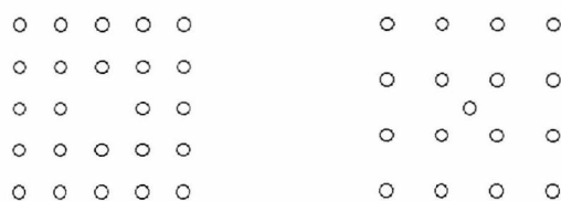
Figure 3.4: A vacancy and an interstitial in a 2D monoatomic solid
