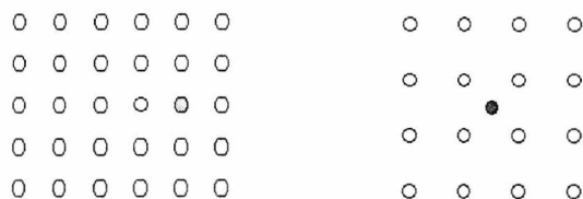
Figure 3.5: A substitutional and an interstitial impurity in a 2D monoatomic solid
