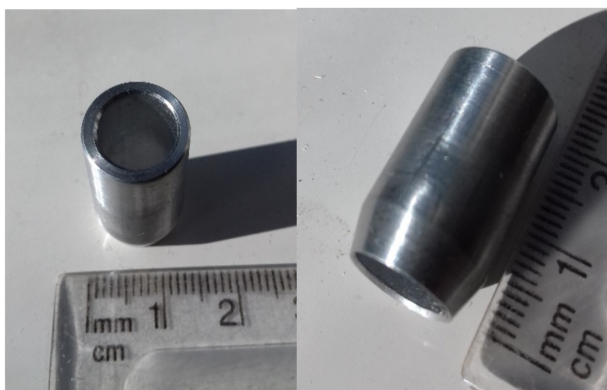
Figure A3.2: Aluminium core (ID 10 mm and height 20 mm) used for soil sampling for neutron tomography.
