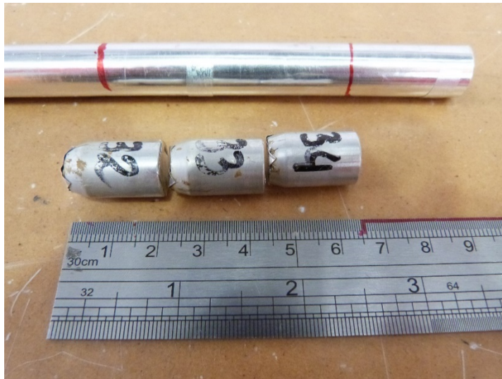
Figure A3.3: Arrangement of three randomly chose soil sample in a cylindrical aluminium sample holder for the scanning.
