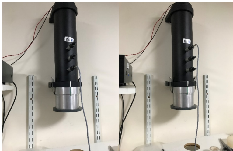
Figure A2.3: Impedance tube measurement by using single microphone in two different positions.
