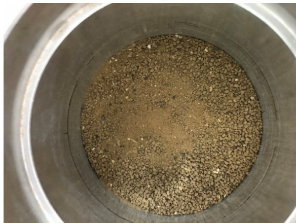
Figure A2.2: Air-dried soil sample repacked in sample holder for impedance measurement.
