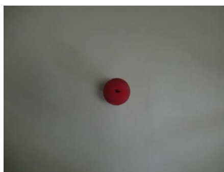
Figure 3: Sensor node placed in the middle of a foam sphere (35 mm diameter and 6 g weight) to represent a table olive Cv. Nocellara del Belice
