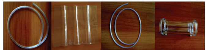
Fig. 1 - PVC pipe, PVC band, TRIFLEX pipe, PC rigid pipe (from left to right).
