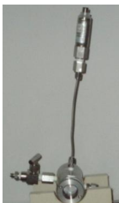
Figure 6.3. View cell adopted for phase behaviour study
