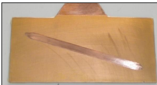
Figure 3.6. Microchannels created in the electrode
