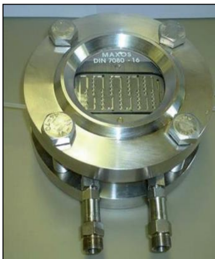
Figure 1.2 Lab-Plate reactor Lonza's Universal Reactor Technology for process development and production.
