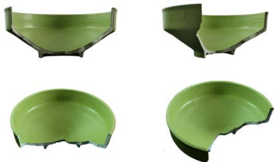
Fig. 14: PLA Model with stucco, polished and colored.
