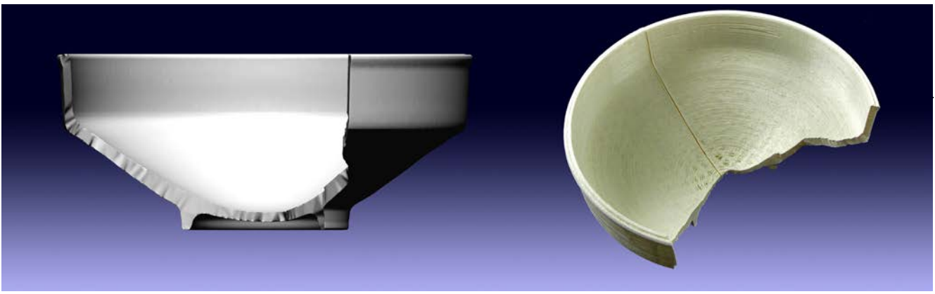
Fig. 16: The model optimized for 3D printing and the PLA model.
