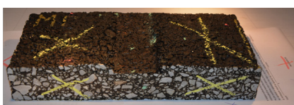
Fig. 3. Rutted sample and marker application.
