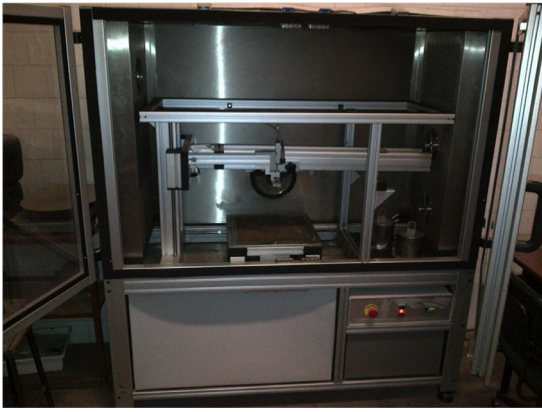
Fig. 2. Wheel Tracker Machine used in DICAM's laboratory.
