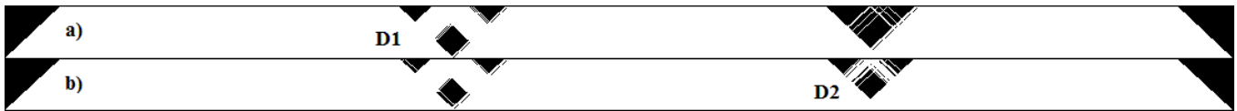
Figure 9: Binarized section images obtained with a threshold value of 40% (a) for D1 and 35% (b) for D2.
