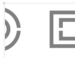
Split ring antennas - A Less Explored Antenna Type in Far Field RFID Tags
