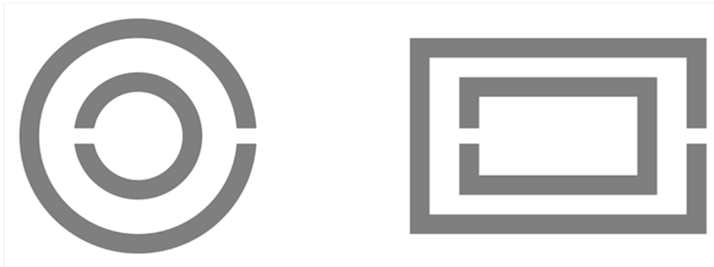
Fig. 2 Common configurations of split ring resonators based on concentric rings and concentric rectangles.
