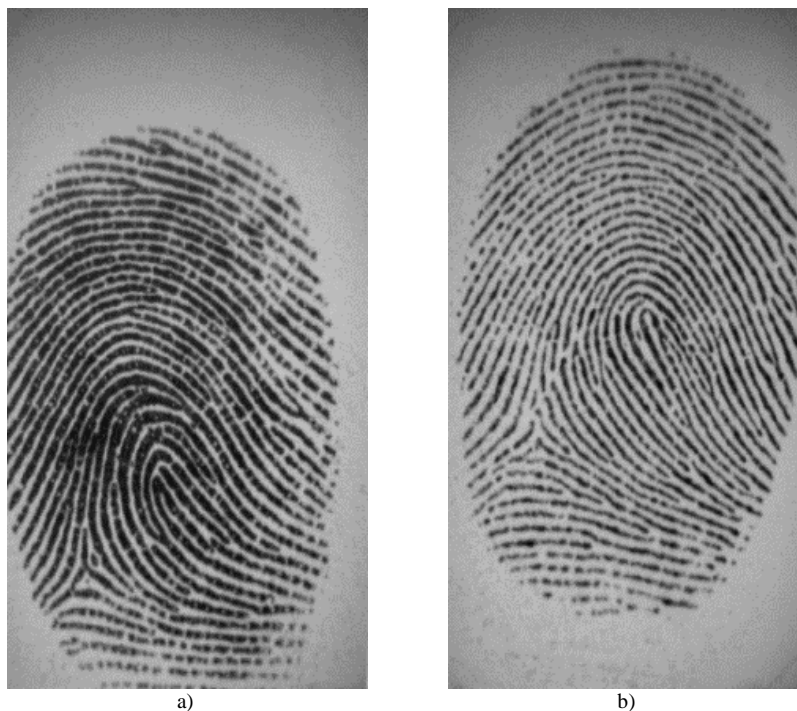
Figure 3.18. Two example images of the FVC2002 DB2-B acquired by Biometrika FX2000 sensor
