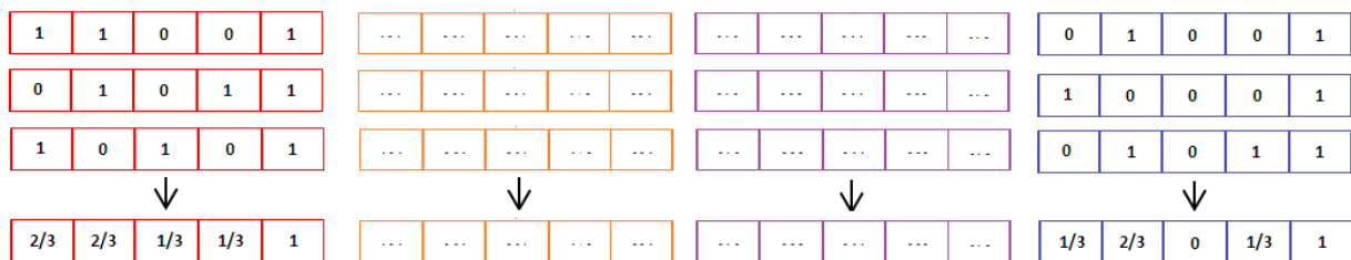
Figure 3.27. The 4 unit centroids obtained applying the average function to the 3 vectors of the same cluster (a different color for each cluster)
