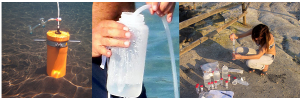
Fig. 3.3- Sample collection system for submarine hydrothermal springs.
