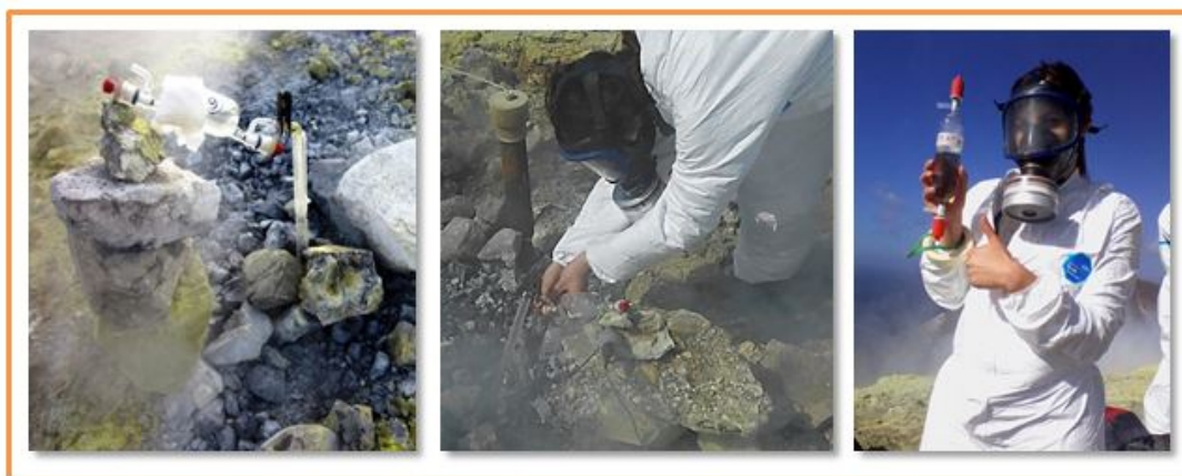
Fig. 3.6 - Sample collection system for fumarolic condensates
