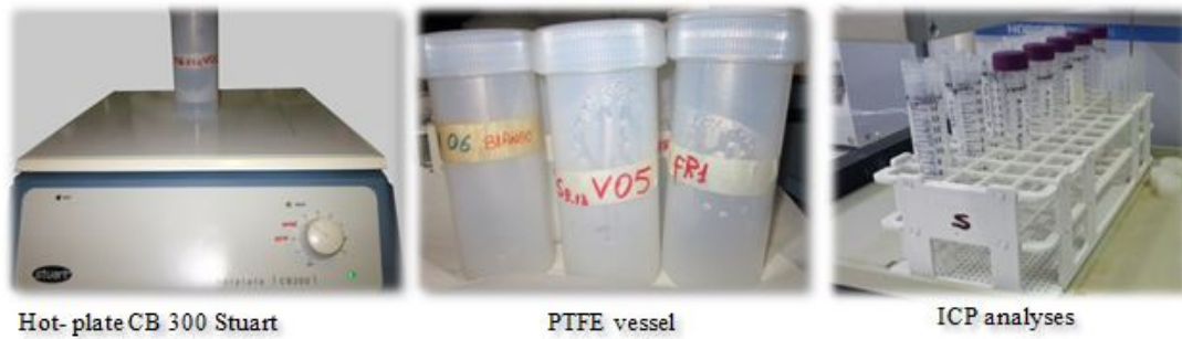
Fig. 3.7- Fumarolic condensates treatment for ICP analyses.
