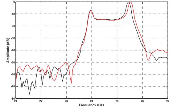
Fig. 6. Experimental results: Stator phase current spectra, under load-varying conditions, for healthy (black) and rotor broken bar (red).
