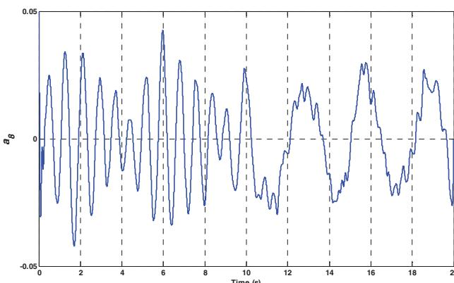
Fig. 10. Wavelet decomposition of  $V_{sl}(t)$ , issued from axial vibration signal, for rotor broken bar conditions, and under load-varying conditions.
