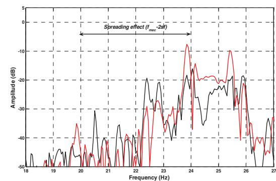
Fig. 7. Experimental results: Rxiial vibration spectra, under load-varying conditions, for healthy (black) and rotor broken bar (red).
