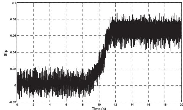
Fig. 4. Experimental results for the used double cage induction motor in faulty conditions, under load-varying conditions. Instantaneous values of slip.
