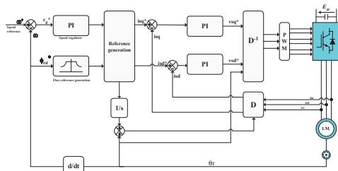
Fig. 1. Block diagram of the control scheme for a typical indirect field-oriented control induction motor drive.
