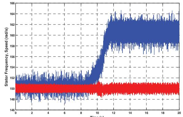
Fig. 5. Experimental results for the used double cage induction motor in faulty conditions, under load-varying conditions. Stator frequency (blue), and speed
