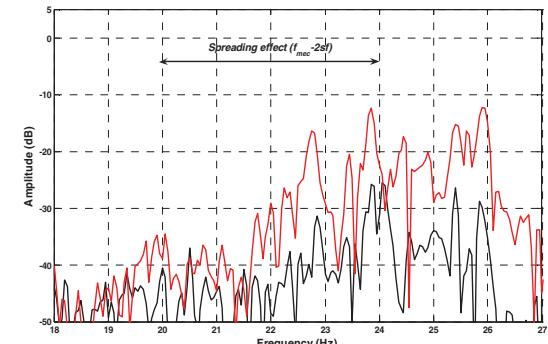
Fig. 8. Experimental results: Axial vibration spectra, under load-varying conditions, for healthy (black) and rotor broken bar (red).
