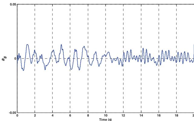
Fig. 9. Wavelet decomposition of  $V_{sl}(t)$ , issued from axial vibration signal, in healthy conditions, and under load-varying conditions.
