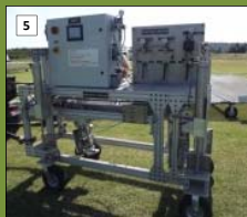
Photos 3-4, Canaway device to measure rotational resistance; Photos 5-6, TAFT device to measure horizontal and vertical force.
