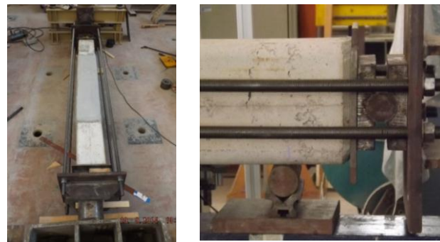
Figure 5. Equipment for the imposition of the constant axial load
