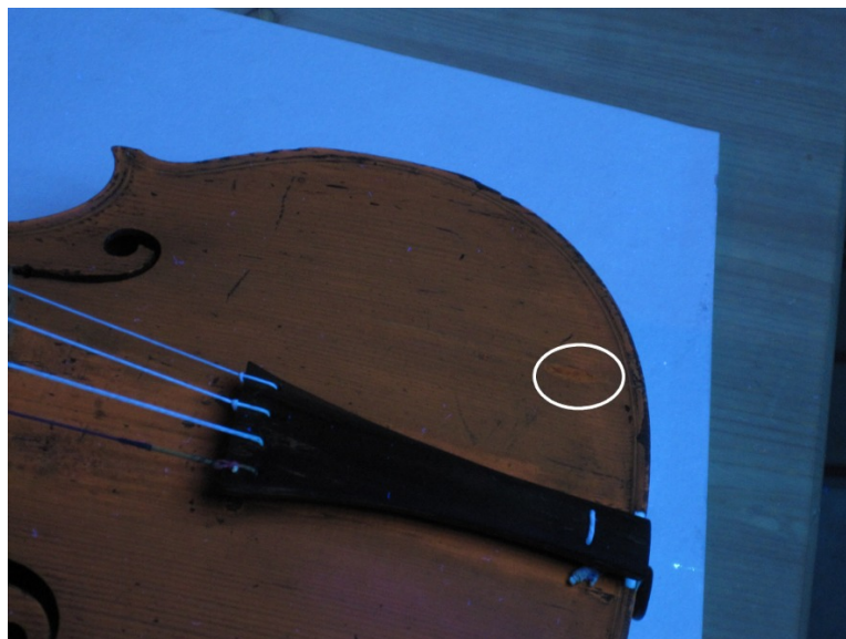
Figure 3.10: Bottom right part of the top of the violin 2781 by B.-J. Boussu illuminated by UV light. The white circle indicates a region with a probable retouch of the varnish. Picture used by permission of the “Musical Instruments Museum”, Brussels.
