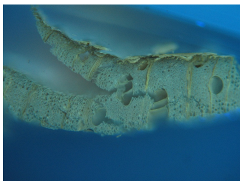
Figure 3.19: Cross section of a portion of the fifth sample from the violin 2002 taken at 100 \times under far blue light.
