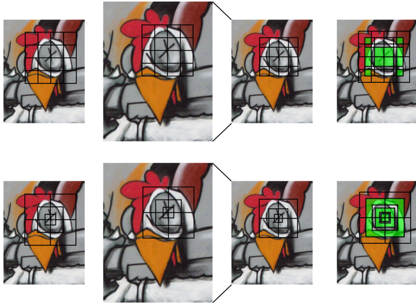
Figure 3.5: A comparison between the SIFT descriptor (top) and the irregular orientation histogram binning (bottom). The descriptors are computed on the original feature patches (first, second columns). By rescaling the second patch (third column) it can be noted a better overlap between cells for the irregular binning method (fourth column). Images from [37]
