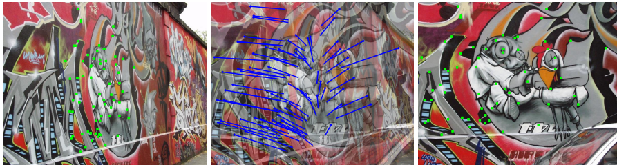
Figure 8.5: A planar homography estimation by the sparse soft matching method. Matched features (green dots) are superimposed on the stereo pair (left, right), and matches are superimposed on both merged images (centre)
