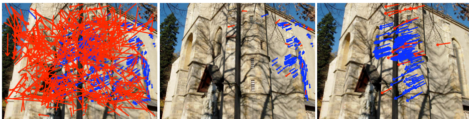
Figure 7.9: Candidate matches (left) with highlighted inliers (blue arrows) and outliers (red arrows). Clustering by the optical flow and taking the first two relevant classes (center, right), it can be noted that almost all elements in the classes are inliers. Images from [124]
