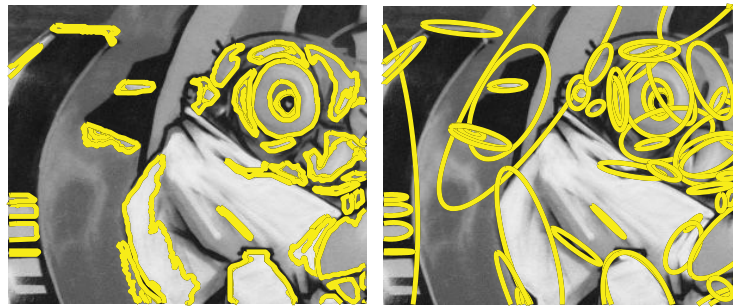
Figure 2.13: Original features detected by the MSER (left) and the associated elliptical patches (right). Image from [177]
