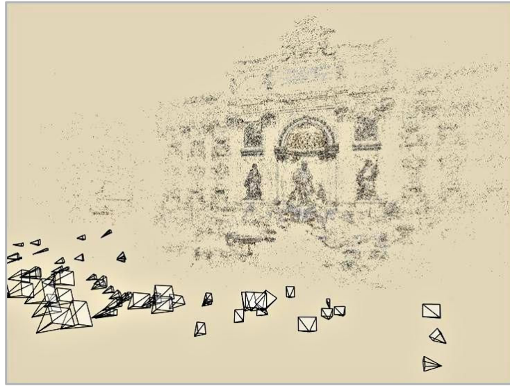
Figure 7.1: A multi view reconstruction of the Trevi Fountain obtained by the Photo Tourism software. Image from [156]
