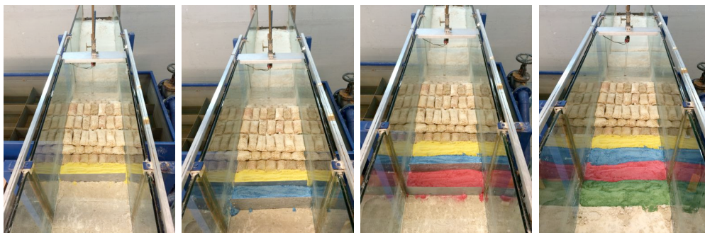
Figure 8 Installation of coloured sand
