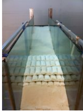
Figure 2 Picture of the geocontainer submerged reef model that was adopted in the present experimental campaign.
