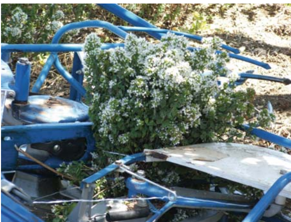
Fig. 18 Mechanization is a necessity for modern essential oil crops growers. In the photo, a prototype of mower modified for harvesting of oregano ( Origanum vulgare L. subsp. hirtum (Link) Letswaart). (Photo: A. Carrubba)
