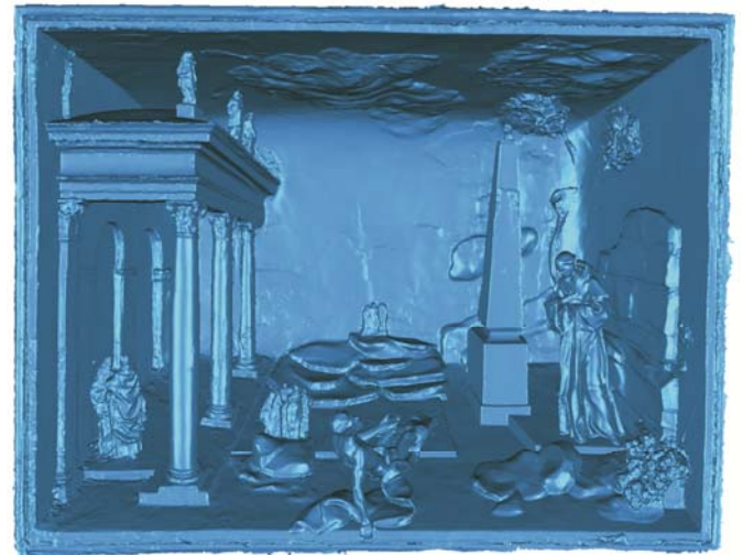
Figure 6: "St. Francis clothes a poor man". Perspective view of the polygon mesh model processed from data acquisition with 3D scanning technique. Interface of the post-processing software Geomagic Studio.
